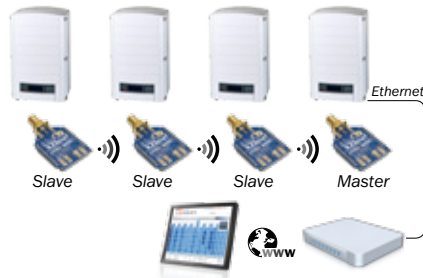
Replacing RS485 inverters interconnections
